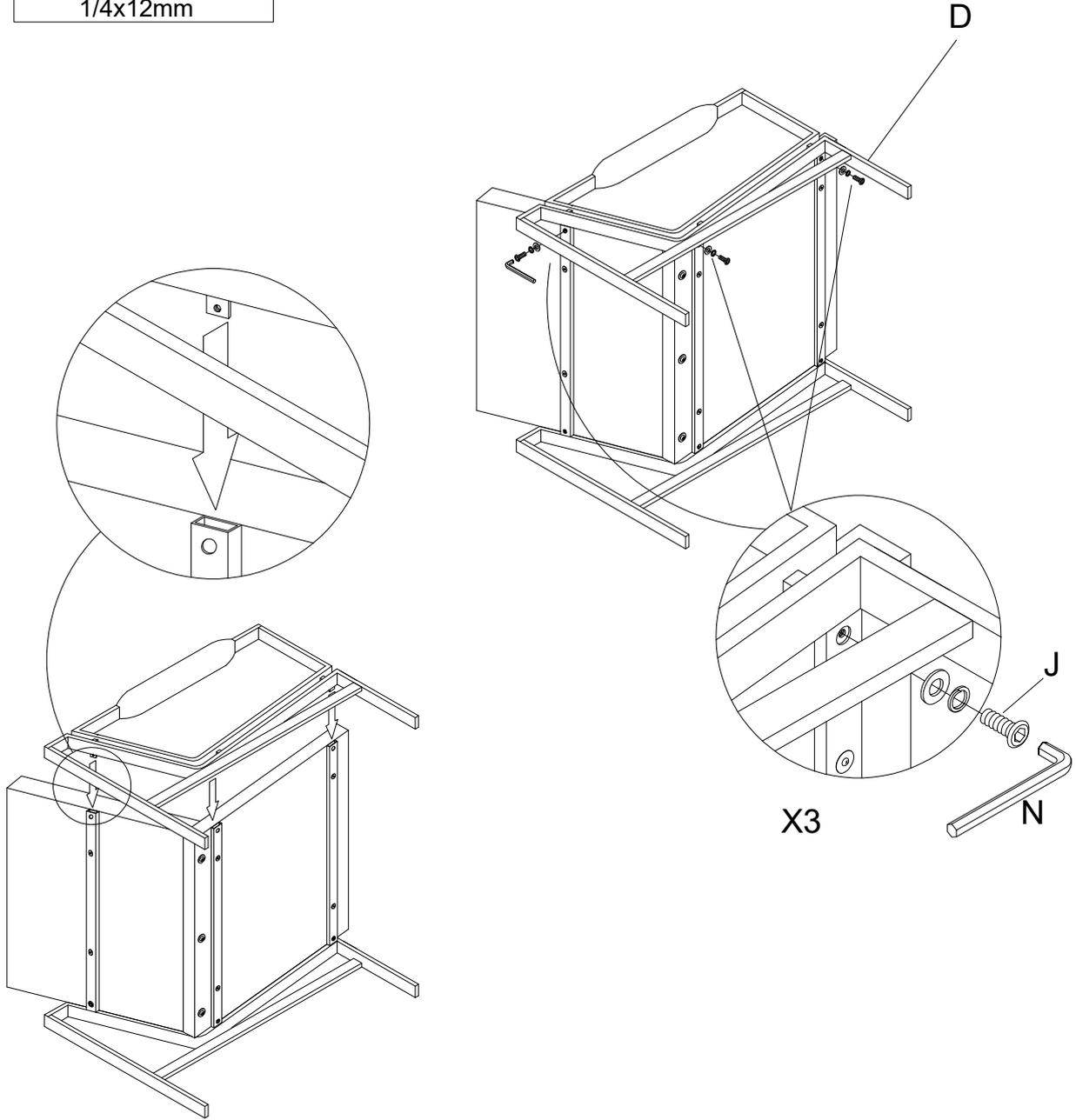
NOTE: Level the chair and tighten all bolts with the allen wrench.
